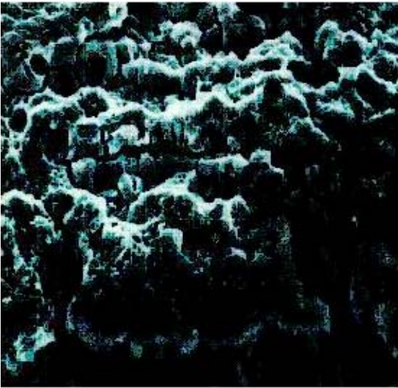
Figure 2-10. Grain Structure of a Corroding Aluminum Surface
